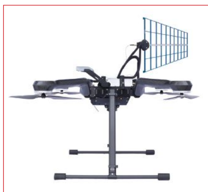
▲ Fig. 1 Integrated drone-based measurement platform.
